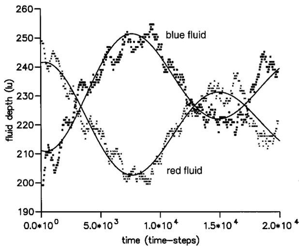
Figure 10. The fluid depth at the centre plotted against time for both the red and blue fluids and the best fit curves through both sets of data when gravity is applied to the heavy particles only, with a strength  $S_g = 0.15$ .
