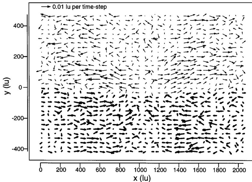
Figure 13. Velocity vector plot for the interfacial internal wave after 10 000 time-steps. Averaging cells containing only or predominantly red particles are represented by the thick arrows. The cells containing only or predominantly blue particles and cells at the boundary containing significant numbers of each particle are represented by the thin arrows.
