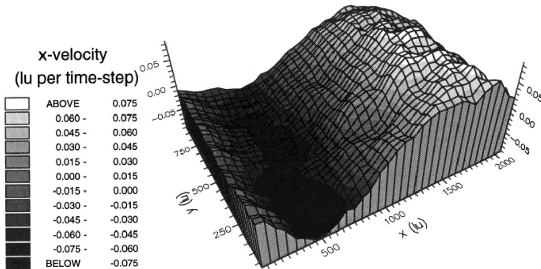
Figure 8. The extrapolated x-velocity distribution of an internal wave in a stratified fluid after 4000 time-steps.
