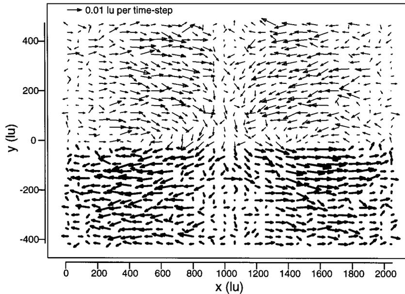
Figure 12. Velocity vector plot for the interfacial internal wave after 4000 time-steps. Averaging cells containing red particles are represented by the thick arrows. The cells containing only or predominantly blue particles and cells at the boundary containing significant numbers of each particle are represented by the thin arrows.
